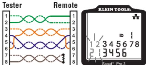
**NOTE:** An open fault or short fault takes precedence over miswires when the appropriate icon(s) illuminates. The Split icon illuminates if the cable wiring does not maintain the designated pairs, an AC signal fault.
