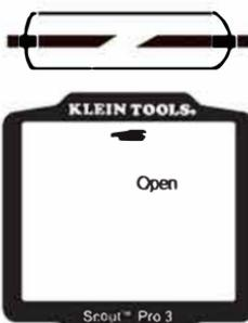
*NOTE: An open fault will also occur when no remote is connected to the satellite end of a video/coax cable.*
