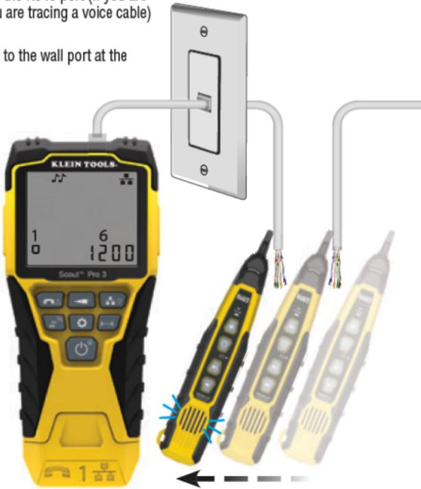
**TONE TRACING ON INSTALLED COAX CABLE (FIG. 8):**
