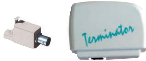
The TC-471 cable tester is a portable instrument whose function is to test the wiring in communication networks.
