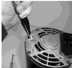
Note: Do not try to turn or rotate the switch until it has been pulled up and is loose.
