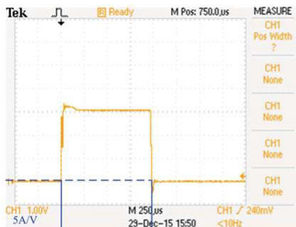
Figure G PEL-5006G-150-600 BMS overcharge flow test program diagram (single pulse)
