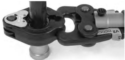
Figure 12A – Placing Actuator Tips Into MegaPress Ring Pockets
