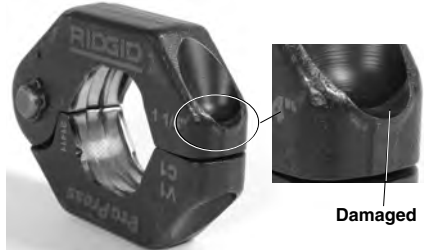
Figure 11 – Damaged Ring Pocket
