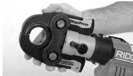
Figure 4 – Sliding The Attachment Out of the Tool
