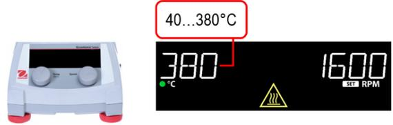
3. To change the heat setting (L) while the heater is on:
