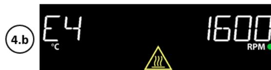
**Note:** To clear an E4 or E7 error code, flip the standby switch (I) off and back on. The unit will be ready for normal use.
