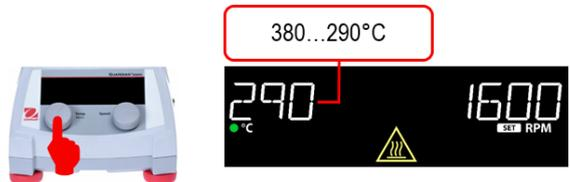
4. To turn off the heater, press and hold the left knob (C) until the unit beeps and the heater indicator (M) disappears.
