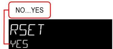
7. Press and hold the left knob (C) until the unit beeps to confirm the Reset setting.
