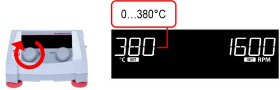
2. To turn on the heater, press and hold the left knob (C) until the unit beeps and the heater indicator (M) illuminates.
