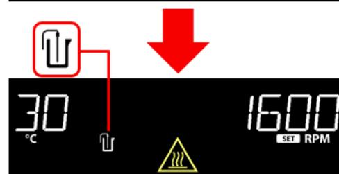
3. If the Ohaus External Temperature Probe is inserted into the external RTD probe port (E) while the heater is running:
