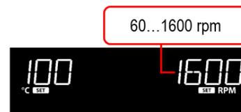
2. To turn on the stirrer, press and hold the right knob (D) until the unit beeps and the stirrer indicator (T) illuminates.
