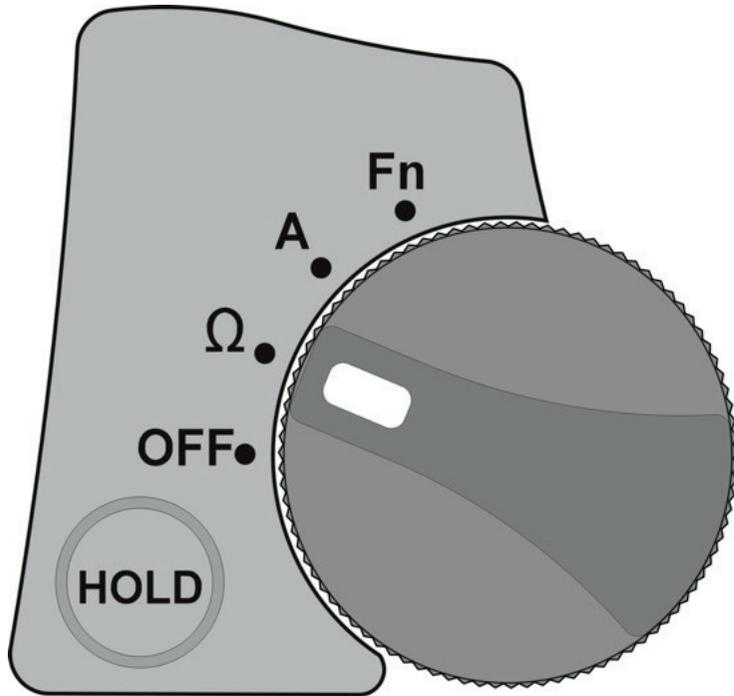
Fig 8. Resistance measurement mode
