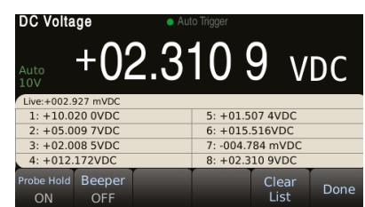
Use probe hold mode to quickly compare a series of readings. Stable readings are captured and added to a list of up to eight measurements.
