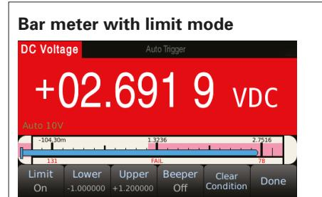
Set upper and lower limit levels with PASS/FAIL counter and indicators.
