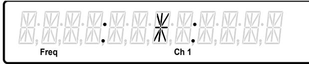
The asterisk (\*) or star represents the measurement and the colons (:) represent the limits you set. This graph indicates that the measurement is within the limits. The colon to the left represents the lower limit, and the colon to the right represents the upper limit.
