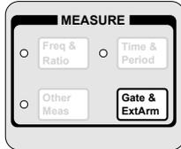
Table 2-2 for the Agilent 53131A (and Agilent 53132A with a serial number prefix below 3646) and Table 2-3 for the Agilent 53132A with a serial number prefix 3646 and above (on page 2-19 and page 2-23, respectively) list the menus for all the arming configurations, and shows how the Gate and External Arming menu changes as a function of the measurement and the arming mode.
