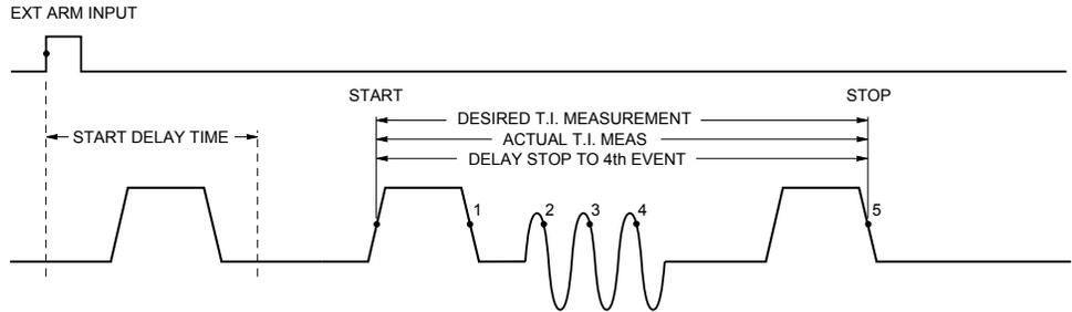
⌘ START: EXT, ⌘ SLOPE: POS, ⌘ DELAY: TIME, ⌘ T: (specified), STOP ⌘: AUTO, DELAY ⌘: EVENT, E ⌘: 5
