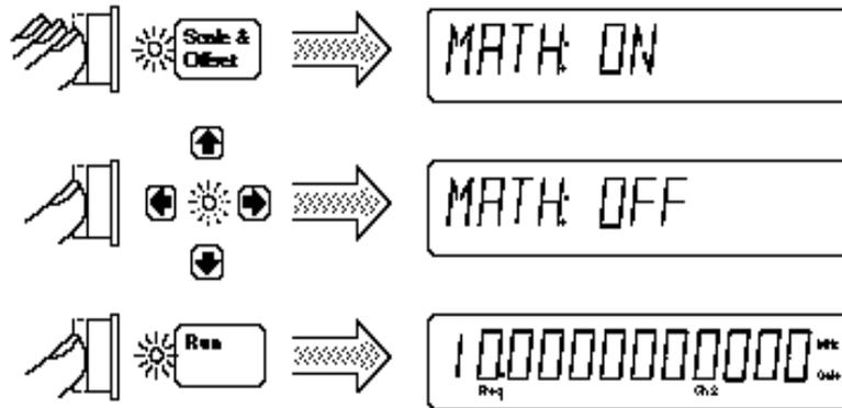
The Counter is now making measurements without the scale/offset values calculated into the measurements.
