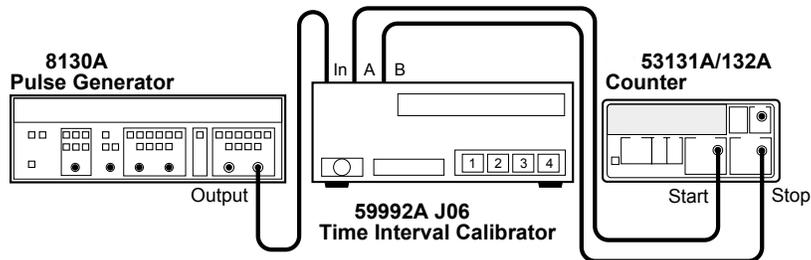
**Figure 2-4. Calibration Setup for CAL: TI FINE?**
