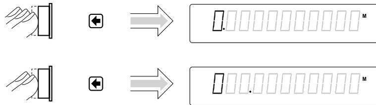
The leftmost “0” digit in the UPPR display is highlighted as shown above, indicating that each press of the d key will increase the displayed value.
