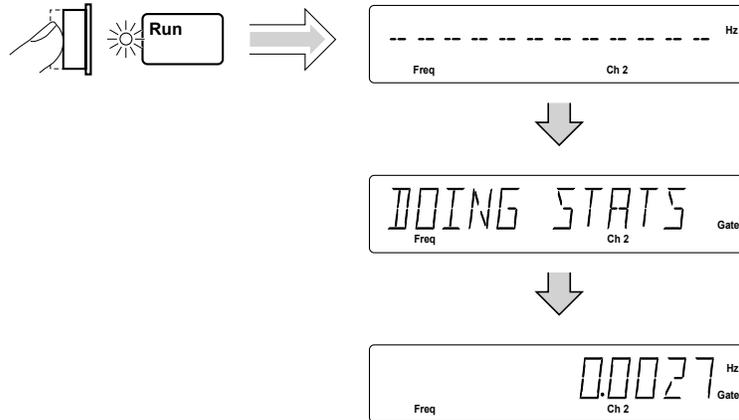
In this case, the displayed standard deviation value is computed on all measurements of the 10 MHz signal since no limits were set.
