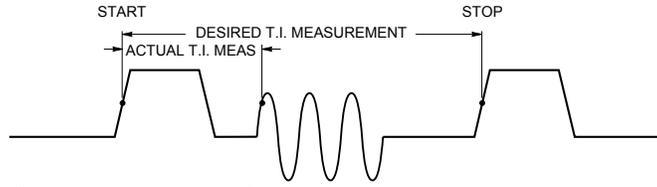
⌘START: AUTO, DELAY ⌘: NONE (standard T.I. measurement)
