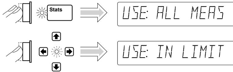
Since the Limits were set to 101 Mega and 102 Mega values that are based on a scale of 10 and offset of 1 Mega, you must re-enable Math now to get the measurements to be within the limits. Perform the following steps.
