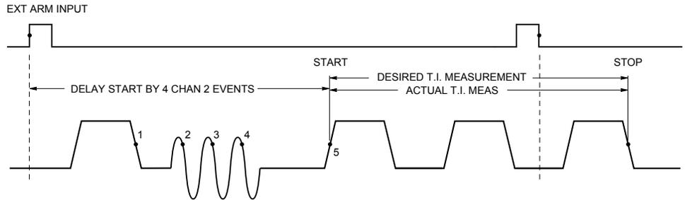
⌘ START: EXT, ⌘ SLOPE: POS, ⌘ DELAY: EVENT, ⌘ E: 5, STOP ⌘: EXT, SLOPE ⌘: NEG, DELAY ⌘: NONE
