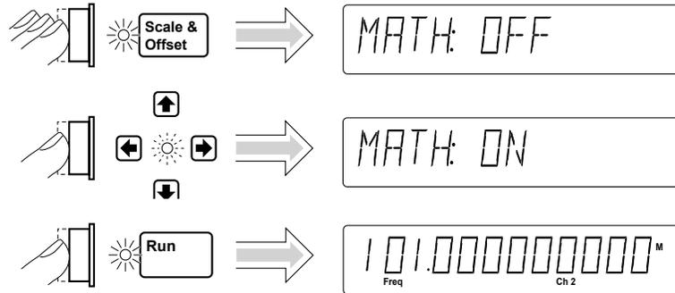
The result of this Math operation is a measurement of 101 MHz.
