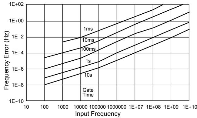
The preceding graphs do not reflect the effects of trigger error. To place an upper bound on the added effect of this error term, determine the frequency error from the appropriate graph and add a trigger error term as follows:
