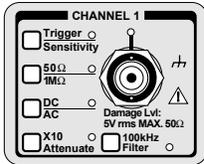
The **Trigger/Sensitivity** keys are menu keys, while the other keys in this group (that is, **50Ω/1 MΩ**, **DC/AC**, **X10 Attenuate**, and **100 kHz Filter**) are toggle keys.
