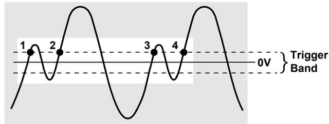
The Counter should now be triggering as determined by the sensitivity level, and displaying the input signal's frequency if the input signal peak-to-peak voltage is large enough for the selected sensitivity level.
