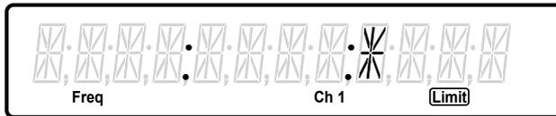
The star is now out of the limits as it has exceeded the entered 10.2 MHz upper limit. (Note the **Limit** annunciator lights since the signal is out of limits.)
