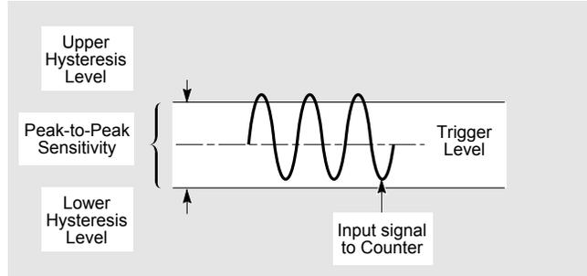
**Signal will not generate a count because the trigger level is set below the midpoint of the signal, causing the lower hysteresis level to not be crossed.**
