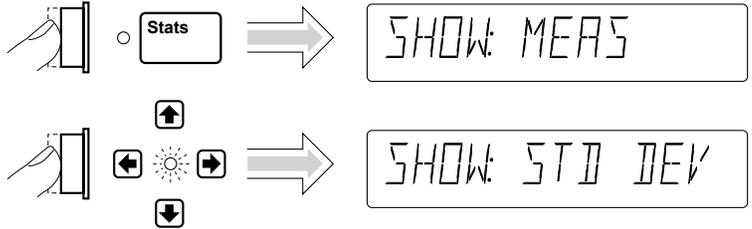
Updating the SHOW configuration caused Stats to be enabled. The Stats indicator is now lit.
