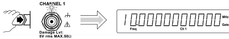
The Counter will automatically display the measured frequency of the input signal.
