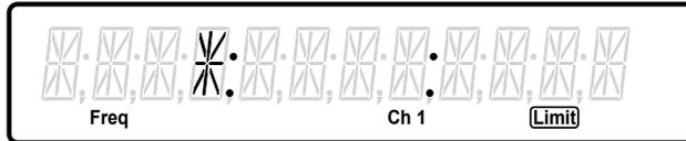
The star is now out of the limits as it is below the entered 9.8 MHz lower limit. (Note the **Limit** annunciator lights since the signal is out of limits.)
