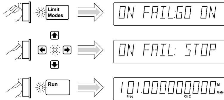
The current modified measurement of the input signal applied to CHANNEL 2 is displayed.
