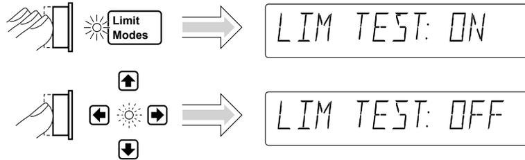
The Counter is now making measurements without limit testing.
