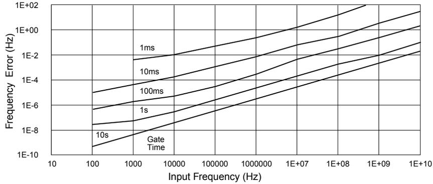
The preceding graphs do not reflect the effects of trigger error. To place an upper bound on the added effect of this error term, determine the frequency error from the appropriate graph and add a trigger error term as follows:
