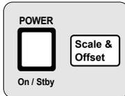
The Calibration menu is accessed by holding the **Scale & Offset** key and cycling the **POWER** key. All of the calibration factors and security settings are stored in *non-volatile* memory, and *do not* change when power has been off or after a remote interface reset.
