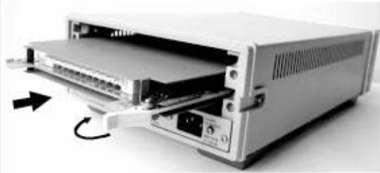
1. Hold the sides of the module, component side **down**, by the metal shields.
