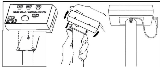
Figure 11. Installing the Combo Tester to the pedestal
