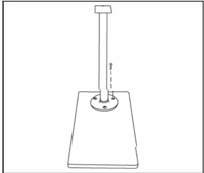
Figure 10. Securing the pedestal to the foot plate
