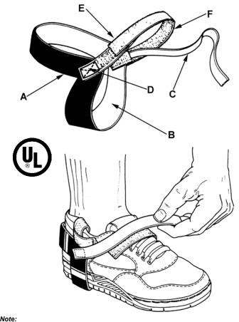
"ESD protective footwear is designed to reduce body charge levels by supplying a
